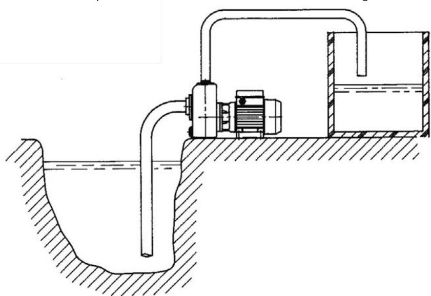
**Fig.3 Circuito aria-acqua in fase di adescamento / Air-water circuit in phase of self-priming**
